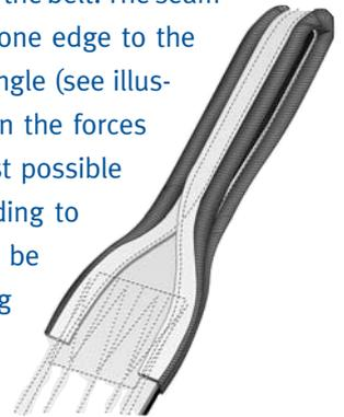
During the straining of a belt the fabric yarns situated in the middle of the belt take the highest strains. For this reason the beginning and the end of the seam must be at the edge of the belt to prevent the seam from opening.
