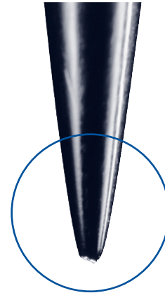
Illustration of a damaged needle point
