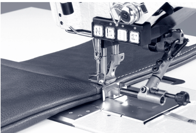
Stitching of a portefeuille-seam (N291-185182) Source: Dürkopp-Adler AG
