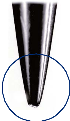
Illustration of a damaged needle point
