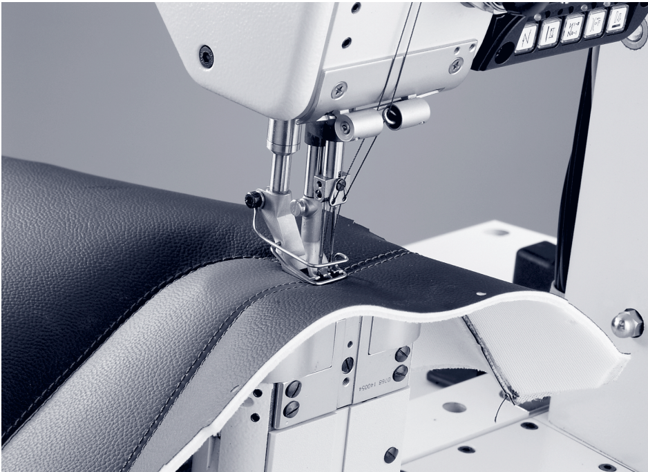
Topstitching of closing seams with a 2-needle postbed machine (768-FA-273-RAP-HP).
