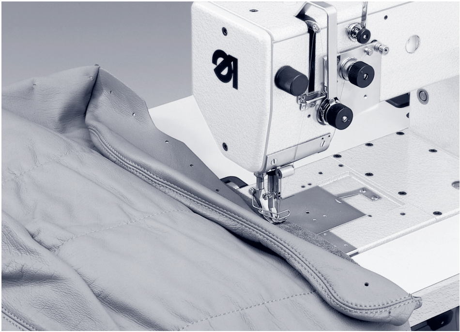
Joining sidewalls to seat plate (767-KFA-373-RAP-HP).
