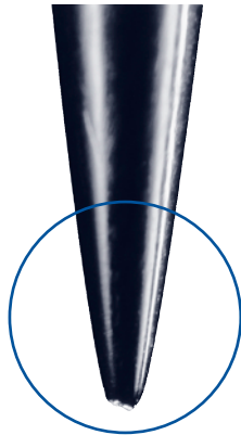
Damaged needle point
